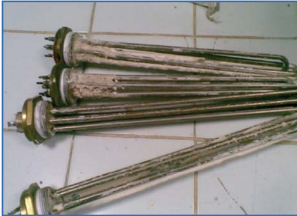
Burst as a result of lime resistance
