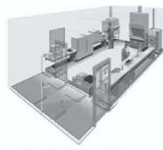
Figure 4. A typical Biosafety Level 3 laboratory (diagram kindly provided by CDC/ATIS, Ft. Detrick, MD, USA). The laboratory is separated from general safety. The air is drawn through an exhaust duct above each work area. An exhaust is available within the facility for the decontamination of equipment or disposal of waste with liquid waste disposal. Special ventilation of air is provided, and all work with infectious materials is conducted within a biological safety cabinet.
